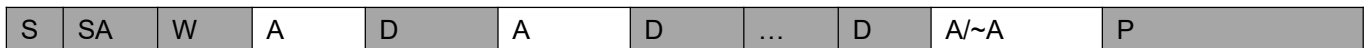
Picture 1.2: The general data format sends from the master device to the slave
